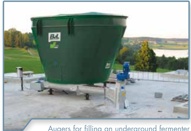
Augers for filling an underground fermenter
