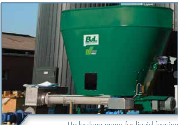
Underslung auger for liquid feeding
